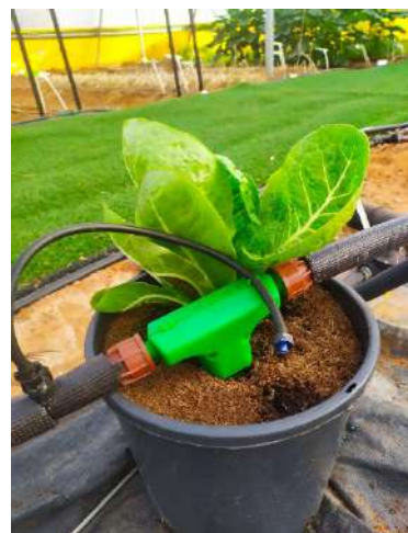
Images: Heat exchange probe coupled with irrigation and fertigation functionality
